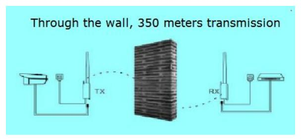
Through the network cable, TX (transmitting) equipment is connected with IPC. RX (receiving) equipment is connected with network cable and NVR or computer, and can be transmitted through a wall within 350 meters.
